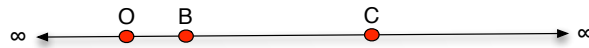
Figure 3.1: On the affine line, the coordinate k of C in the coordinate frame [O, B] is k = OC/OB .
