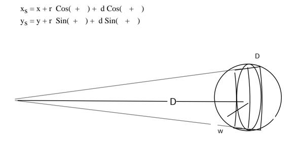
Figure 2.3 Model of the Ultrasonic Range Sensor and its Uncertainties
