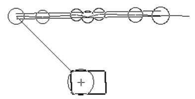
**Figure 4.2a** A vehicle (rectangle with cross) with an circular uncertainty in position of 40 cm (circle surrounding cross) is shown detecting a line segment. The top image shows a set of range data in which a line segment has been detected. The projections of ultrasound readings are illustrated as circles of radius  $_{\rm W}$ . The projections provide the vertices of the sonar horizon. The detected segment is illustrated by a pair of parallel line at  $\pm$  c.
