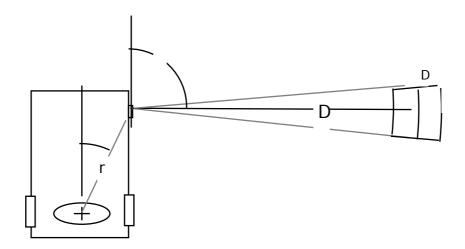
Figure 2.2 Projection of a Range Reading to External Coordinates
