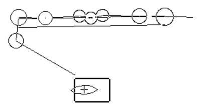
**Figure 6.2** This figure shows the uncertainty in position after correction by matching with model segment number 0. The uncertainty is reduced to an ellipse with a minor axis of approximately 8 cm. An error of (x, y) = (20 cm, 20 cm) had been introduced to the estimated position before the segment was detected. Following matching, both the position of the robot and the observed segment have been shifted by y = 17.7 cm by the update process to correct for the error.
