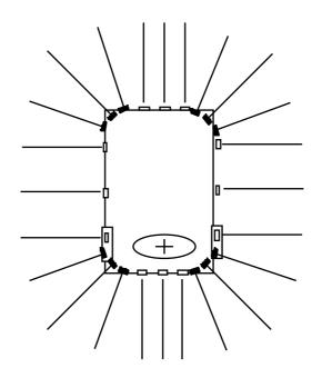
Figure 2.1 Configuration of 24 Ultrasonic Range Sensors
