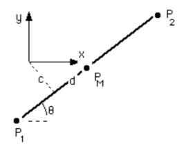
Figure 3.1 The Parametric Representation for a Line Segment.
