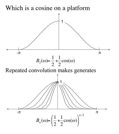
The binomial coefficients provide a series of low pass filters with no ripples.
