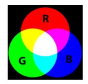
The RGB model "pretends" that Red, Green and Blue are orthogonal (independent) axes of a Cartesian space.
