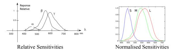
Cones provide our chromatique "day vision". Human Cones employ 3 pigments : Short Wavelength: cyanolabe  $\alpha$  400–500 nm peak at 420–440 nm Medium Wavelength: chlorolabe  $\beta$  450–630 nm peak at 534–545 nm Long Wavelength: erythrolabe  $\gamma$  500–700 nm peak at 564–580 nm
