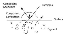
For Lambertian reflection, the intensity || P(i,j) || is generally determined by changes in surface orientation, while color is determined by Pigment.
