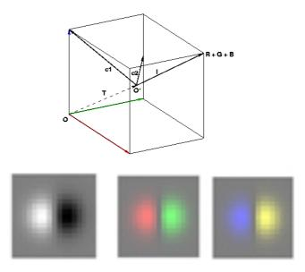
Such a vector can be "steered" to accommodate changes in ambient illumination.
