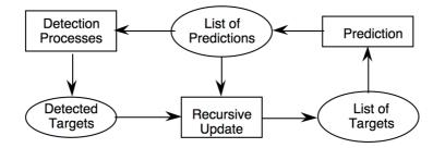
The detection process can contain errors due to missed detection and false detection. To minimize the influence of errors we use the idea of a Gaussain window.
