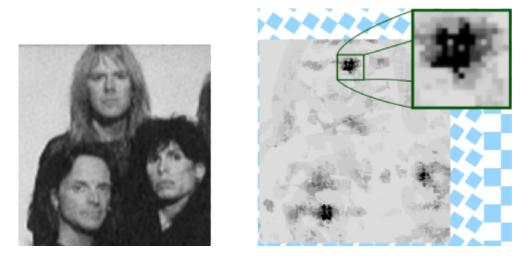
Faces can be detected as the center of gravity of "deep" detections. Faces can be tracked using the Bayesian tracking described in the previous session.
