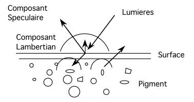
Most reflectance functions can be modeled as a weighted sum of two components: A Lambertian component and a specular component.
