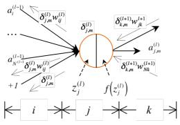
We compute error terms,  $\delta_j^{(l)}$  for each unit *j* in layer *l* back to l = l - l using the sum of errors times the corresponding weights times the derivative of the activation function.
