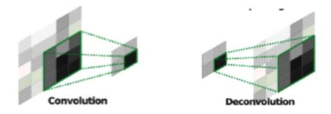
De-convolution treats the learned receptive field as basis functions, and uses the activation at level l to create a weighted sum of bases at level l+1.
