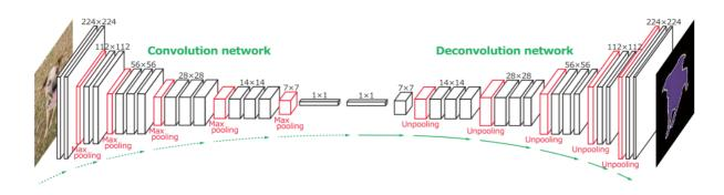
VGG uses max pooling. With Max pooling, unpooling requires remembering which unit was selected for each pooling operation. This is done with a "switch Variable" that records the selected unit. The output is a larger sparse layer in which 3/4 of the activations are zero.
