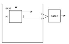
A sliding window detector is a brute force method to test if a pattern can be found in an image. This approach was made popular by the Viola-Jones face detector, now found in most smart phones and tablets. A typical architecture for a sliding window detector looks like this:
