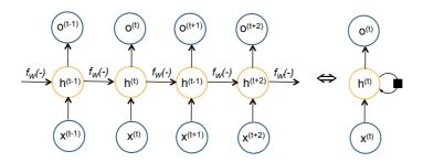
Where the black square represents a time delay of 1 time unit. The recurrent structure can be unfolded to see the network as a 2-D structure.
