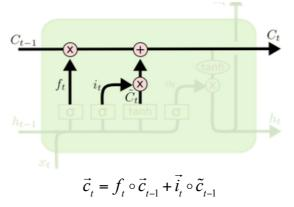
The cell state is then updated by multipling the previous state by ft to determine how much to forget (attentuate) the previous state, followed by the addition of the new state  $c_t$ .
