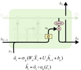
The output is then based on the a filtered version of the cell state, A sigmoid layer which decides what parts of the cell state to output. This is then modulated by a *tanh* to set scale the value between -1 and +1.
