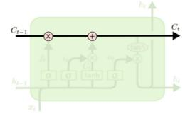
The horizontal line running through the top of the diagram represents the cell state. The cell state is kind of like a conveyor belt. It runs straight down the entire chain, with only some minor linear interactions. It's very easy for information to just flow along it unchanged.
