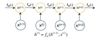
The temporal duration of the network is typically represented the variable  $\tau$ , so that the network is said to operate on a temporal sequence  $x^{(t)}$  from t=1 to  $\tau$ .
