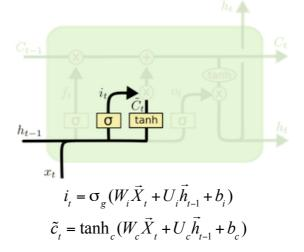
This has two parts. First, an "input gate layer" uses a sigmoid to determine which values to update. Then, a tanh layer creates a vector of new candidate values,  $\tilde{C}$  t that may be added to the state.
