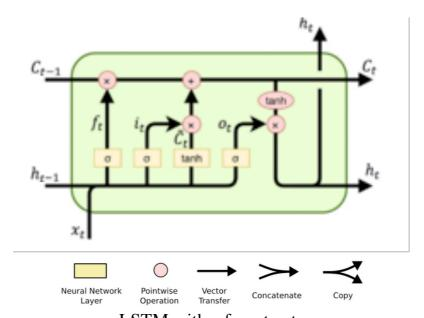
LSTM with a forget gate
