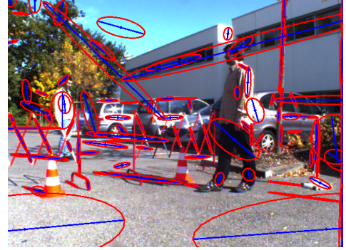
Fig. 2. An example of Scale Invariant Ridge Segments detection. Each detected segment is represented by an ellipse where the main axis represents the position of the segment and the second axis represents the scale.
