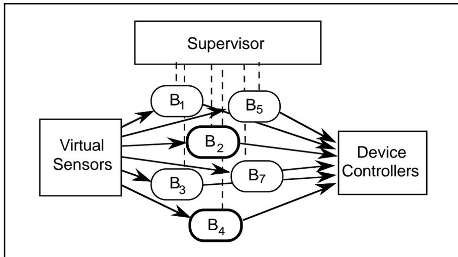
**Figure 1** . A Supervisory controller selects and controls the sequencing of perceptual processes (shown as B for Behaviours). Multiple processes can be active at the same time. Arrows indicate flow of data, dashed lines indicate control, the highlighted ellipses are currently active.
