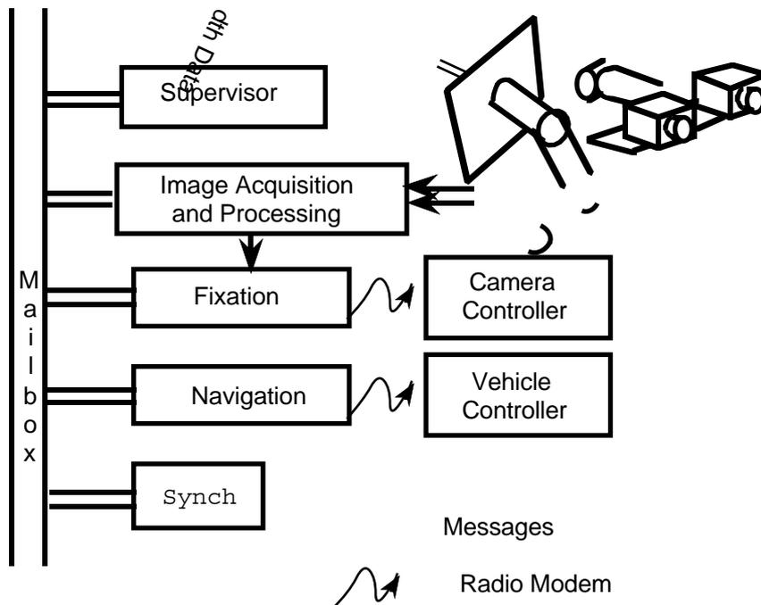
Figure 3 Configuration of demonstration system within the SAVA III Vision test-bed.
