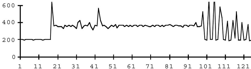
**Figure 4.** Timing diagram for image acquisition and processing from a typical tracking session. Vertical axis is milli-seconds. Horizontal axis is cycle number.
