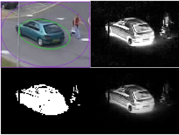
Figure 6: Failed split (test sequence 1, p = 2 , frame 589). Clockwise, the images depict the video, D , D \times \text{MASK} , and D' .
