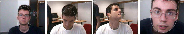
Figure 1. Example of face tracking. First and second moments provides an ellipse which delimits the face in the image
