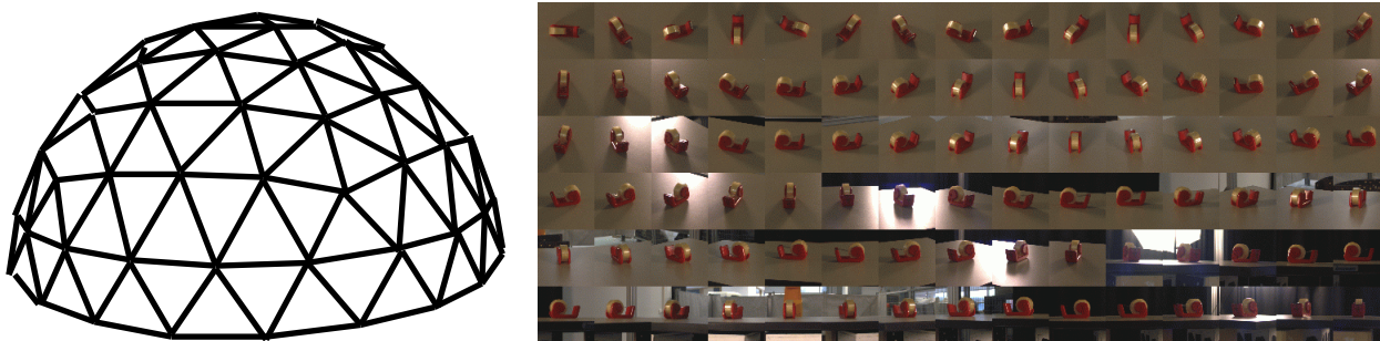
Figure 9. A geodesic sample function for the view sphere defined by a Geodesic dome with a spacing of R/10 . The half sphere contains 91 images. On the right a set of 90 images sampled with a geodesic function.
